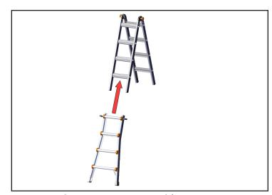
4. Insert the new inner assembly into existing outer assembly.
