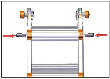
5. Re-engage lock tabs to lock the outer assembly to the inner assembly.
