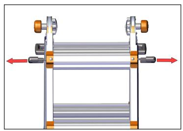
Pull out lock tabs to disengage outer assembly from inner assembly.
